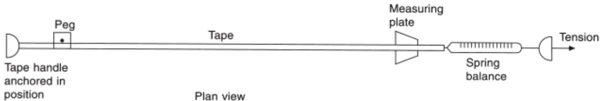
2. Using a linen tape, arrows are aligned between the two points at intervals less than a tape length. Measuring plates are then set firmly in the ground at these points, with their measuring edge normal to the direction of taping.
